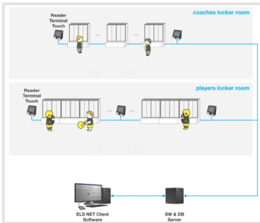
The software designed by Metra enables each player access to their own personal locker by selecting their profile and entering their pin code on one of the touch-pad displays. This system also allows for control by staff from a central server removing the need for locker keys and making changing locker assignments at the end of the school year more efficient.
